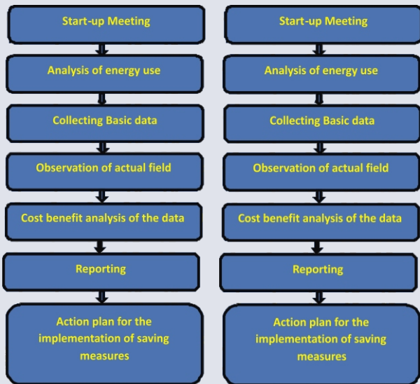
Fig. 1. flowchart for proposed methodology for energy audit
